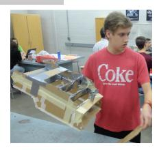
The hopper is constructed out of welded sheet metal. The front extension, however is 1/16" polycarbonate. The extension is fastened with pop rivets and automotive tape.
