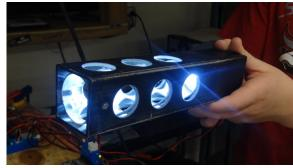
flashlight is powered through a spike, then through a 12V-5V converter to dim the light. The light only turns on when we are aiming at the goals to avoid shining it in drivers' eyes.
