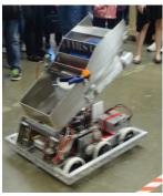
The shooter is designed to make 3-Point shots from behind the Pyramid. These shots can be taken from either the center or corners of the Pyramid.
